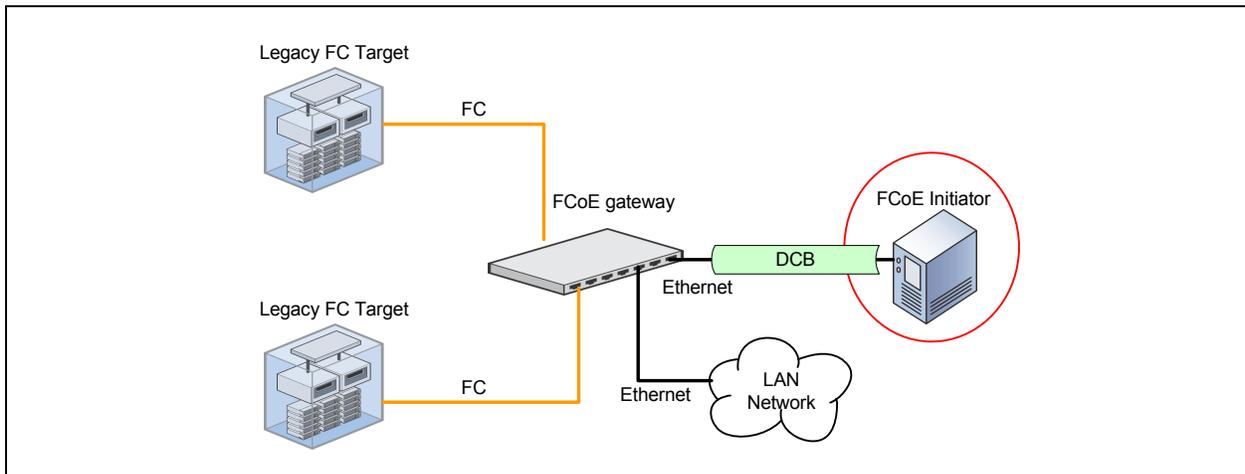
**Figure 7.47. Connecting an FCoE Initiator to FC Targets**
