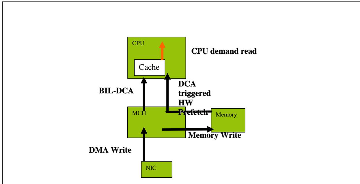
**Figure 7.29. Diagram of DCA Implementation on FSB System**
