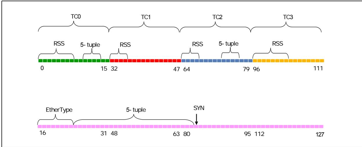
Figure 7.5. Example of Rx Queue Allocation (Non-Virtualized)
