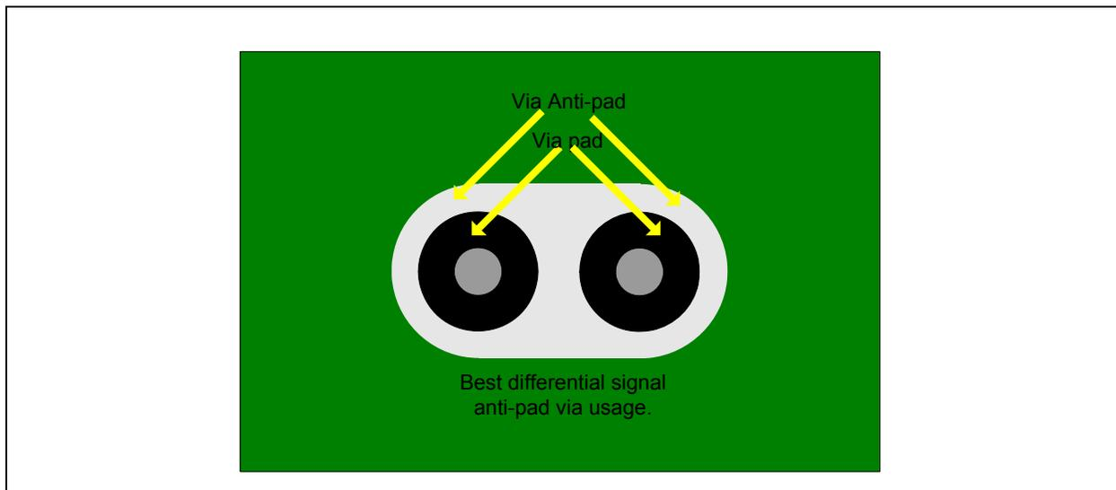
Figure 12-15. Best Differential Signals Via Anti-Pads
