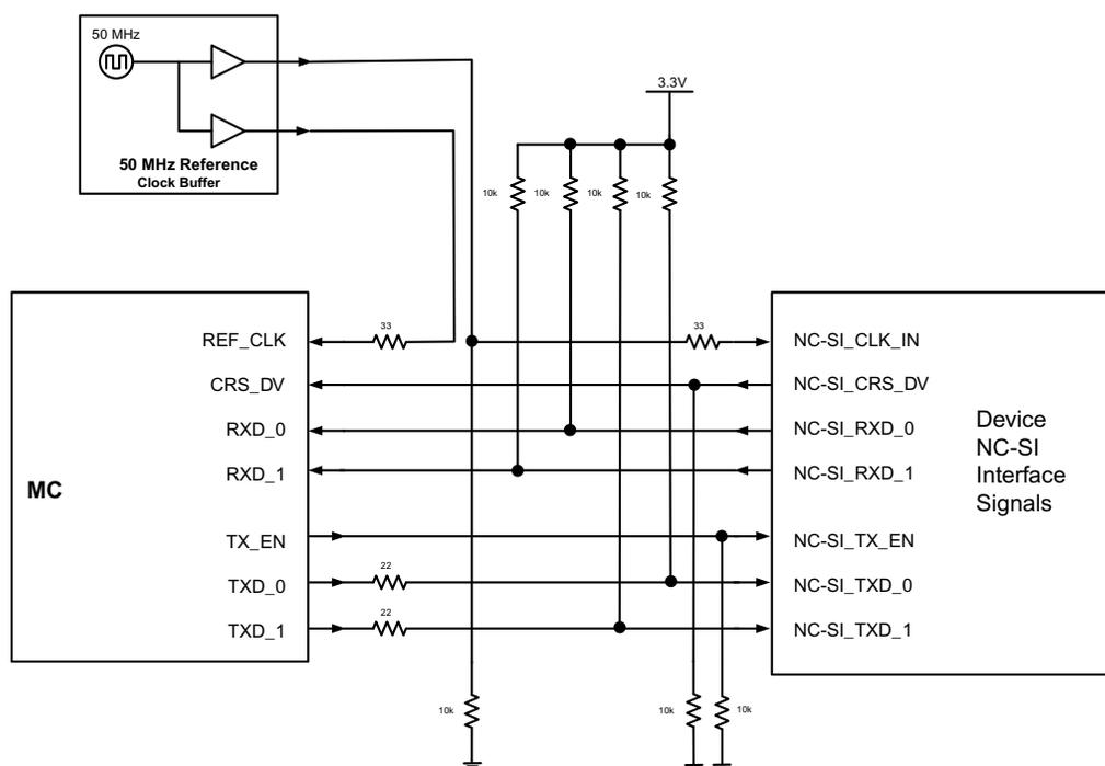
Figure 12-19. NC-SI Connection Schematic: Single-Drop Configuration
