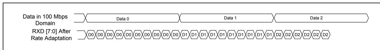
**Figure 3.18. Data Sampling in 100 Mb/s Mode**
