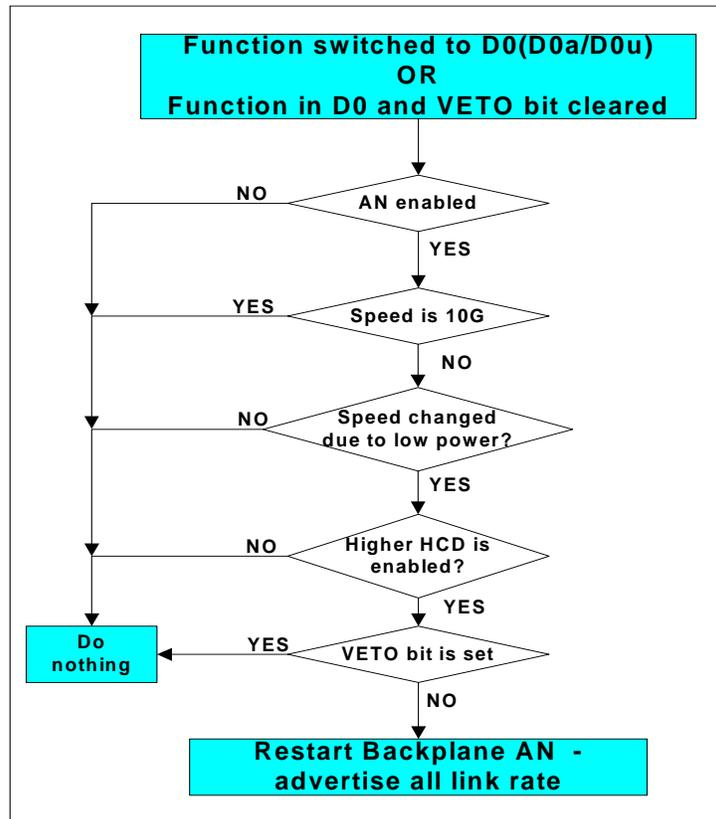
Figure 3.27. MAC Speed Change on Entering Power-up Mode
