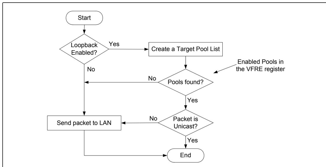
Figure 7.41. Tx Filtering
