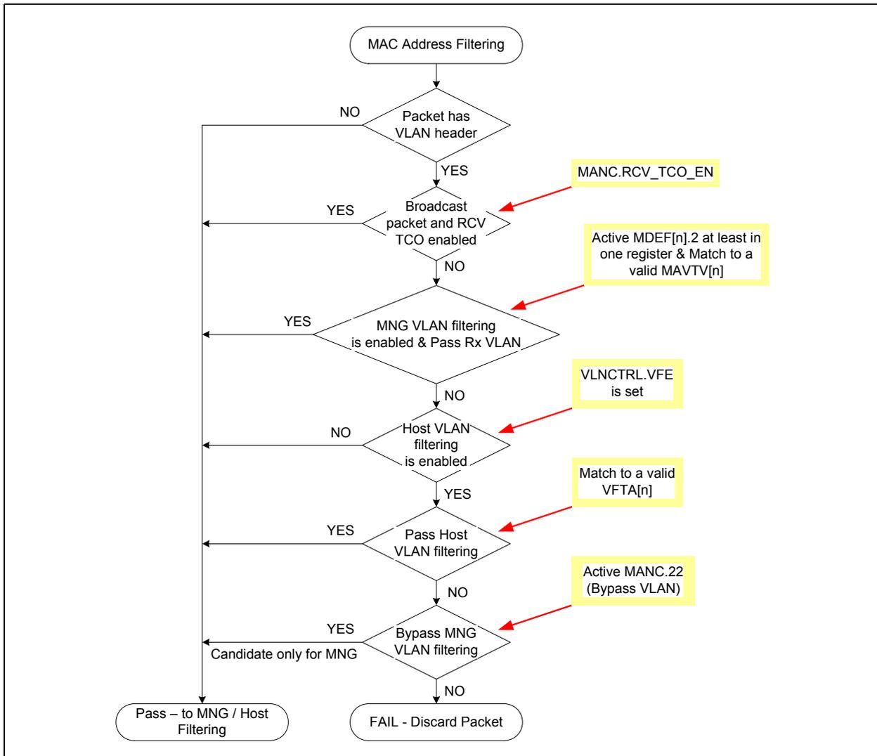
Figure 7.3. VLAN Filtering
