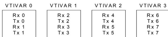
**8.3.5.2.8 VF Interrupt Vector Allocation Registers — VFIVAR\_MISC (0x00140; RW)**
