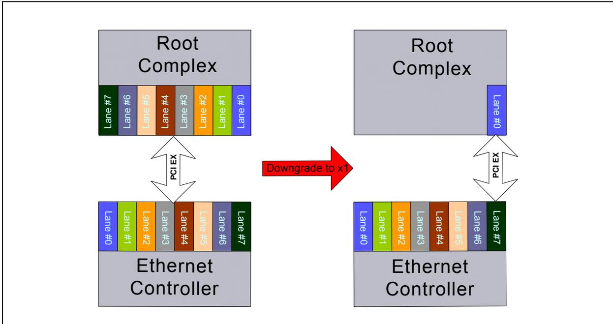
Figure 3.3. Lane Downshift in a Reversal x8 Configuration
