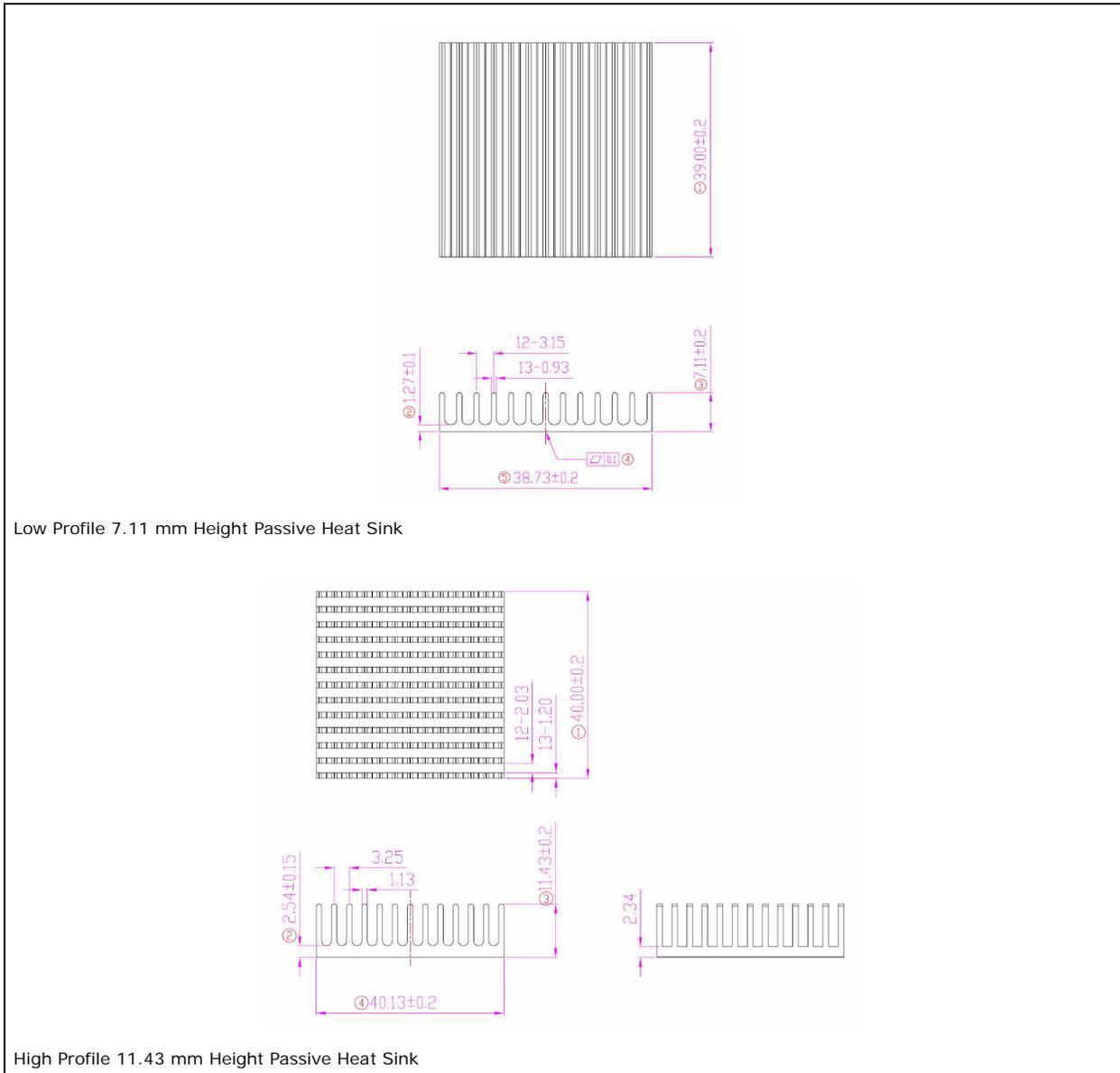
Figure 13-4. Extruded Heatsinks
